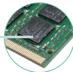
● Apacer DRAM module with conformal coating
